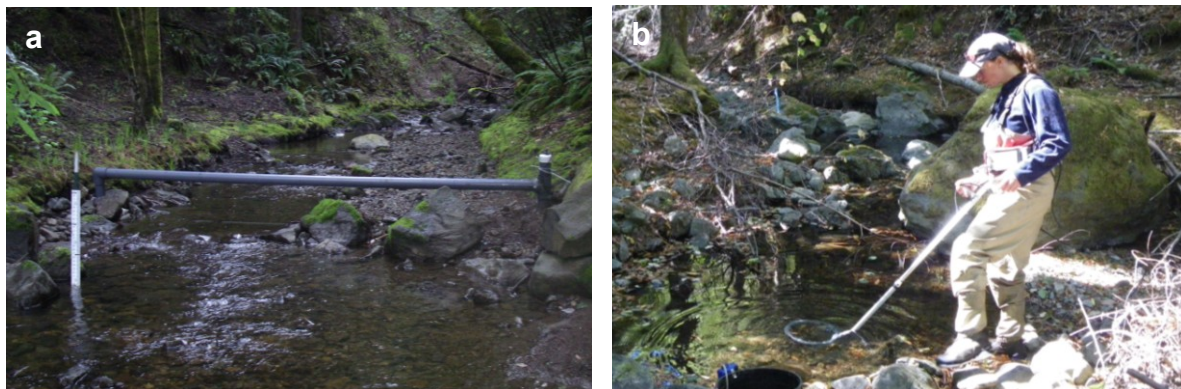
Figure 5. Stationary (a) and portable (b) PIT tag detection systems used to detect movement and presence of PIT tagged coho in study reaches.
