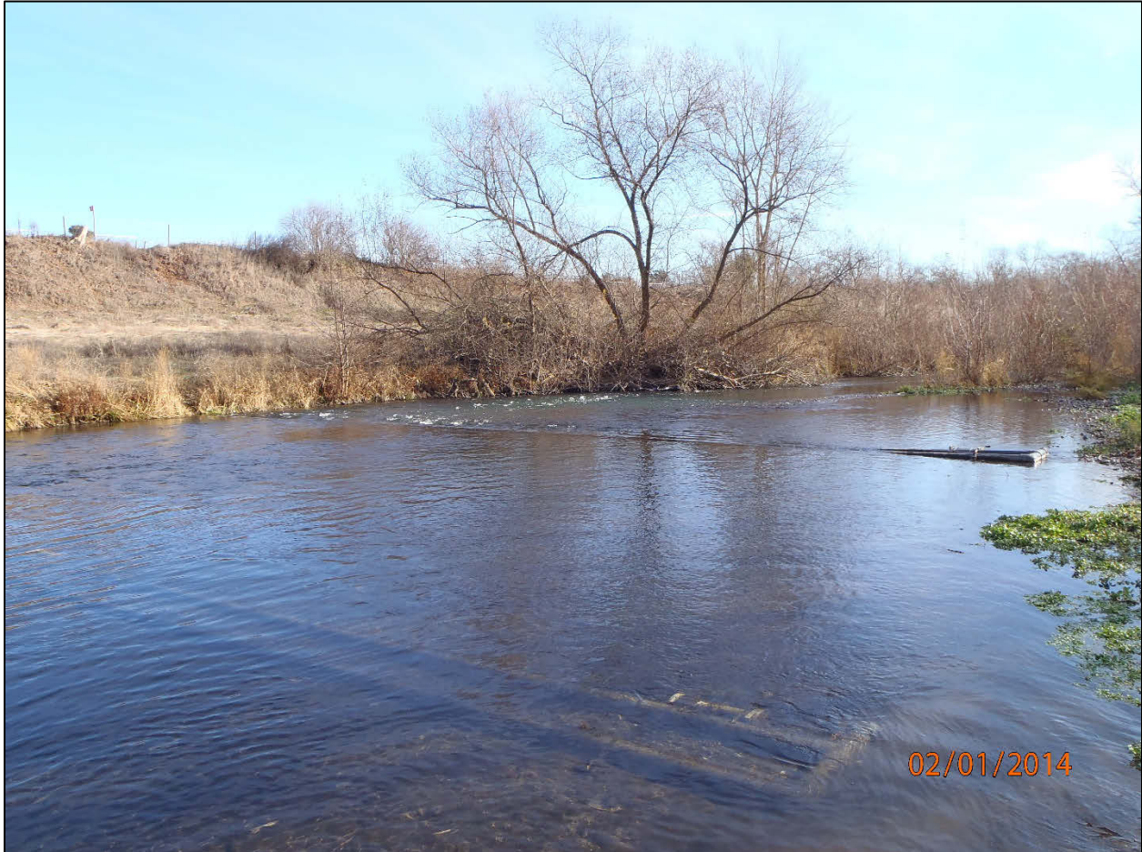
Figure 4. Paired, flat-plate PIT antenna array near the mouth of Dry Creek (rkm=0.36). Array consists of an upstream set of three antennas and a downstream set of three antennas. Individual antennas within a set are 20 feet long and anchored to the stream bed such that each set spans the wetted width of Dry Creek during all but high winter flows.
