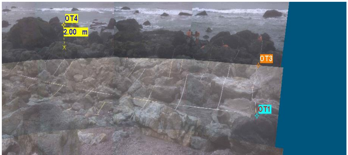
Figure 37. Stitched photomosaic of Pyramid Point (PYR). Locations of survey bolts are marked.
