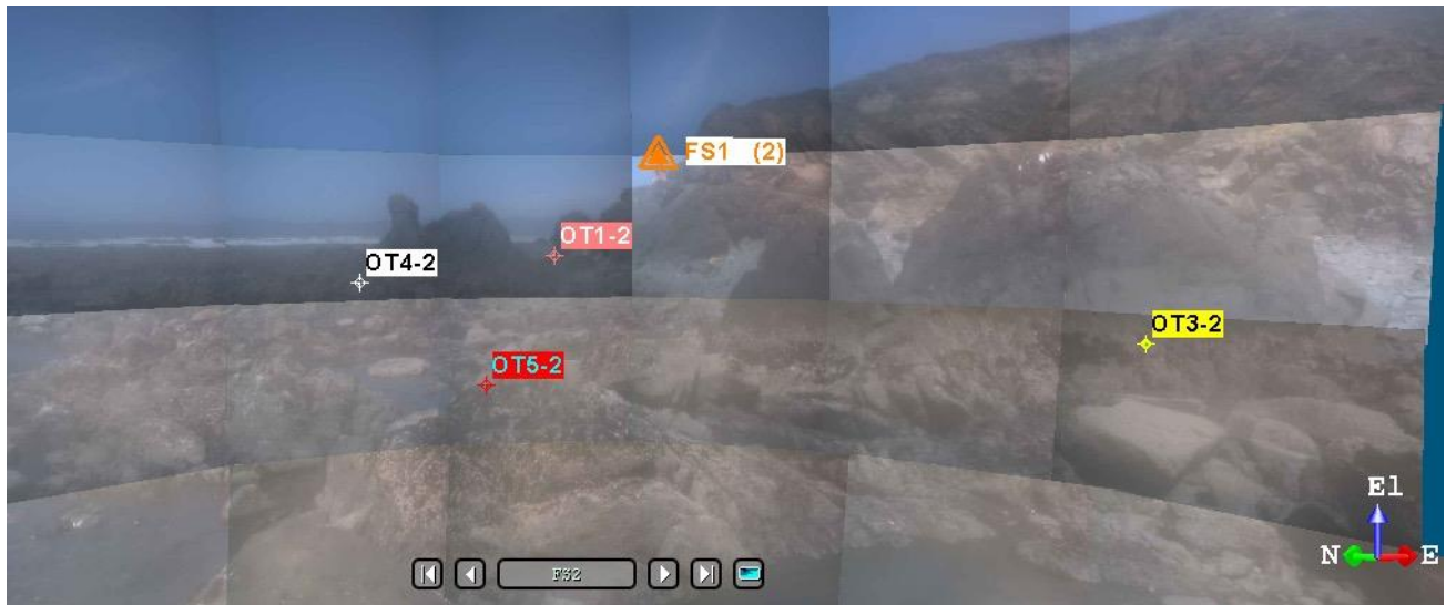
Figure 33. Stitched photomosaic of Point Saint George (PSG). Locations of survey station and bolts are marked.
