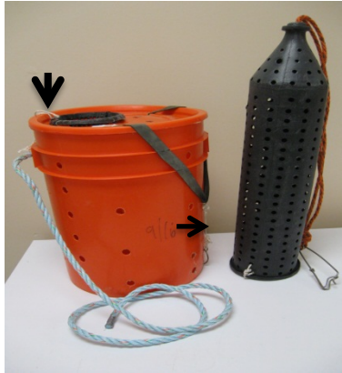
FIGURE 1. —Standard Korean-style trap (right) with 6.4-mm holes and an 18.9-L bucket trap (left). The trap on the left is an example of one of the 16-mm hole diameter test traps. Note the cotton twine, as indicated by the arrows, which serves as the destruct device.
