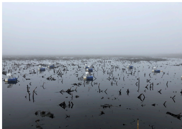
Automated chambers for greenhouse gas measurements, installed in a corn field during a fallow season flooding event.
