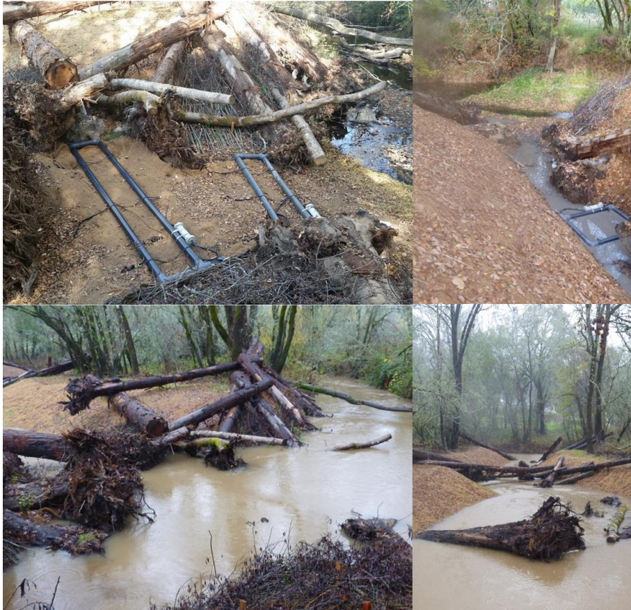
Figure 4. Off-Channel PIT antenna sites prior to winter flows (top) and after the habitat was activated (bottom). The off-channel inlet array, GRE-6.09, is on the right and the off-channel outlet array, GRE-6.03, is on the left.
