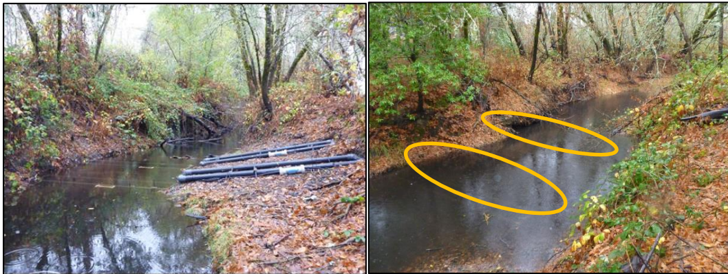
Figure 3. PIT antenna arrays in the main channel of Green Valley Creek upstream and downstream of the proposed side channel inlet and outlet. GRE-6.13, a four-antenna array, is on the left. GRE-6.01, a two-antenna array (antennas circled), is on the right.
