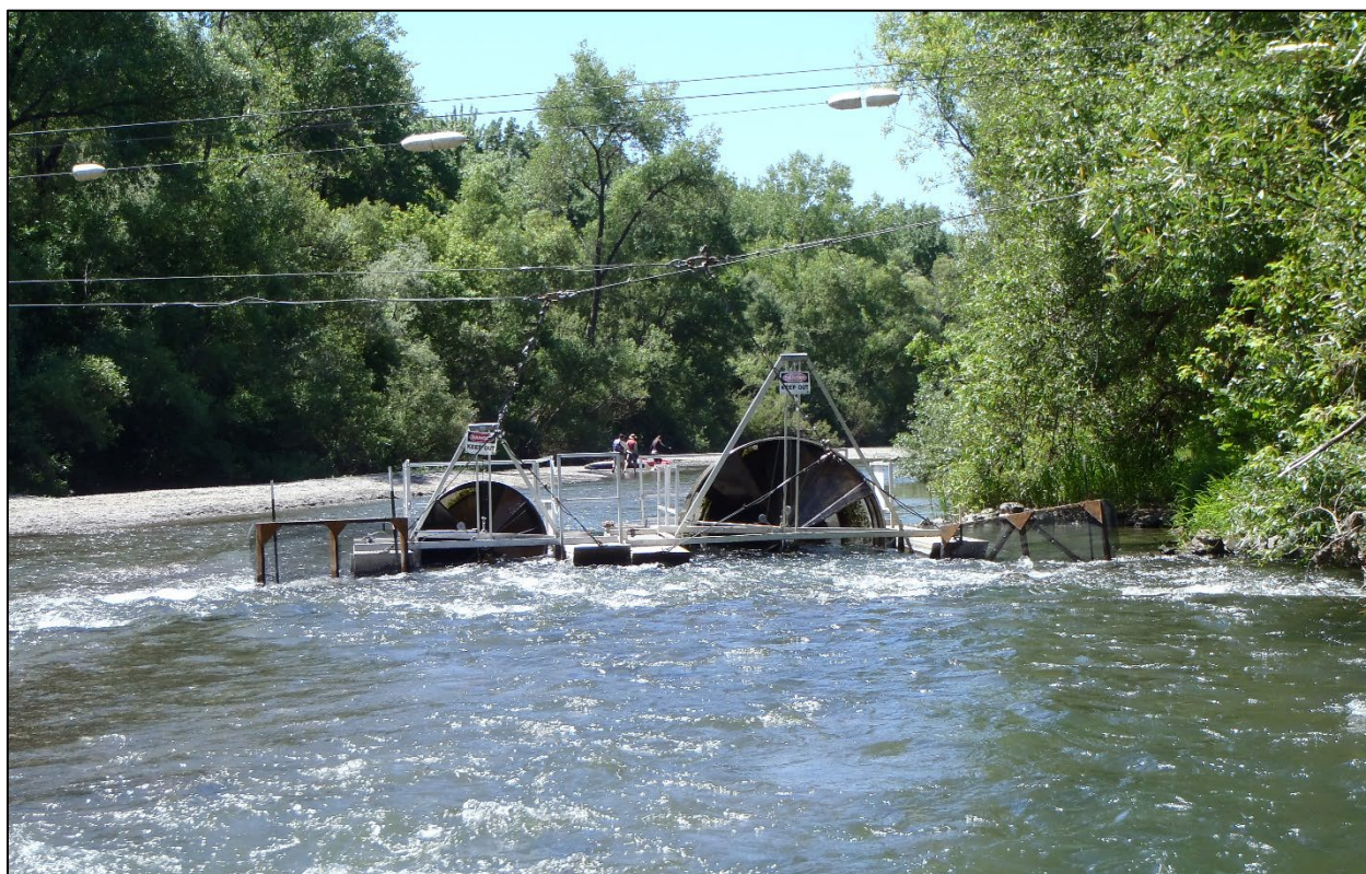
Figure II-2. Downstream migrant traps at Sonoma Water's Mirabel dam in Forestville (Chinook smolt LCS, rkm 39.67).
