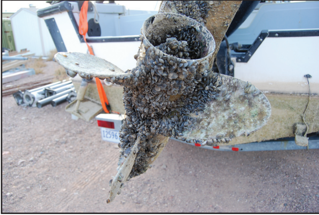
Figure 11. Boat propeller encrusted with quagga mussels. Photograph courtesy of the National Park Service.
