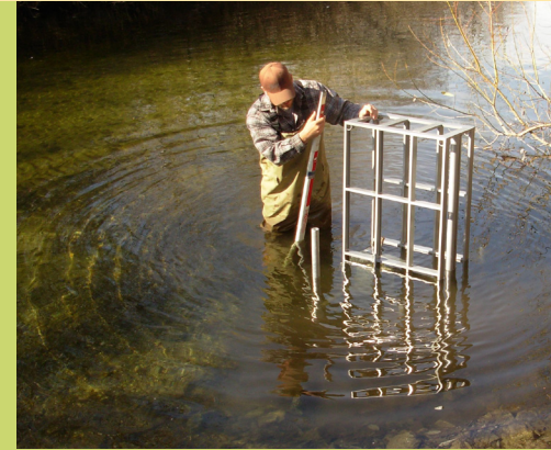
Monterey Peninsula Water Management District staff deploy sonar camera on the Carmel River. Monterey Peninsula Water Management District.
