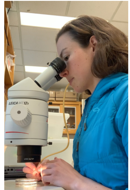
Laboratory culture experiment set-up. (top) Fischer uses a microscope and mouth pipet to isolate cells of the dominant marine and freshwater diatom genera, Thalassiosira and Entomoneis , from upper San Francisco Estuary water. (bottom) Many weeks later, these isolated cells have grown into robust cultures. Photos: Alexis Fischer.
