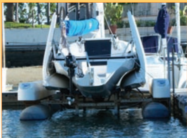
Boat lift isolates hull from water
