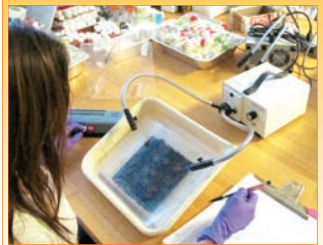
Counting fouling organisms using grid placed over experimental panel
