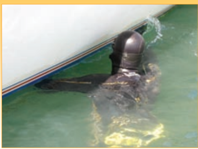
Diver uses a soft pad to clean boat hull in water
