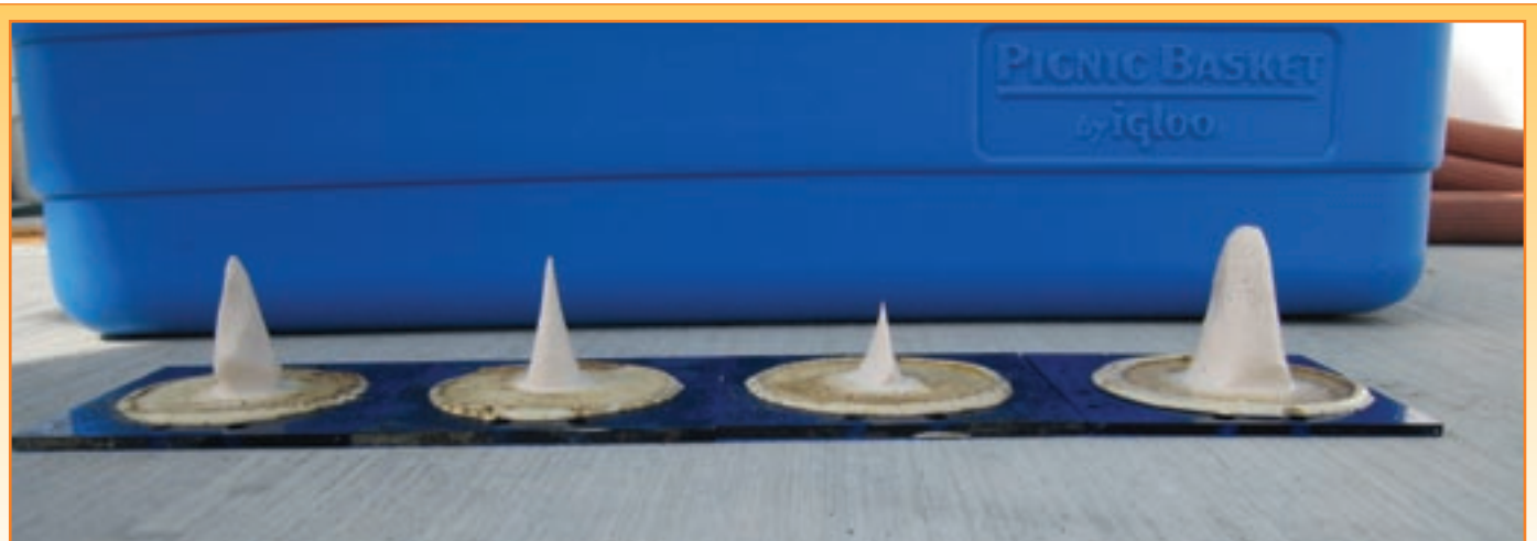
SLODS™ cards measure water flow
