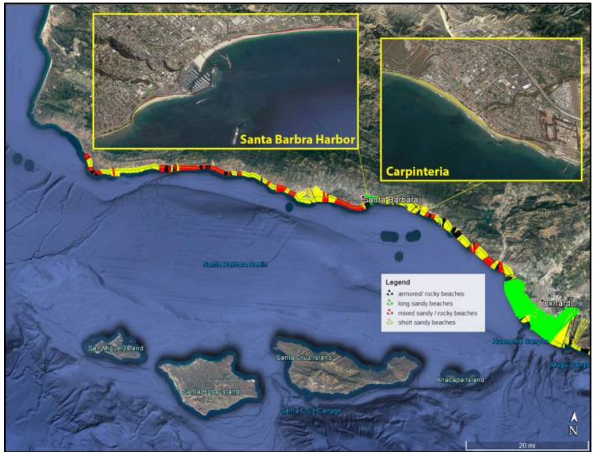
Figure 4.6. CoSMoS-COAST model domain for Santa Barbara County. Green transects indicate long sandy beaches; yellow transects represent short sandy (“pocket”) beaches; red transects represent mixed sandy/rocky beaches; and black transects represent harbors and armored or cliffed beaches. Future shoreline projections are shown for Santa Barbara Harbor and Carpinteria.
