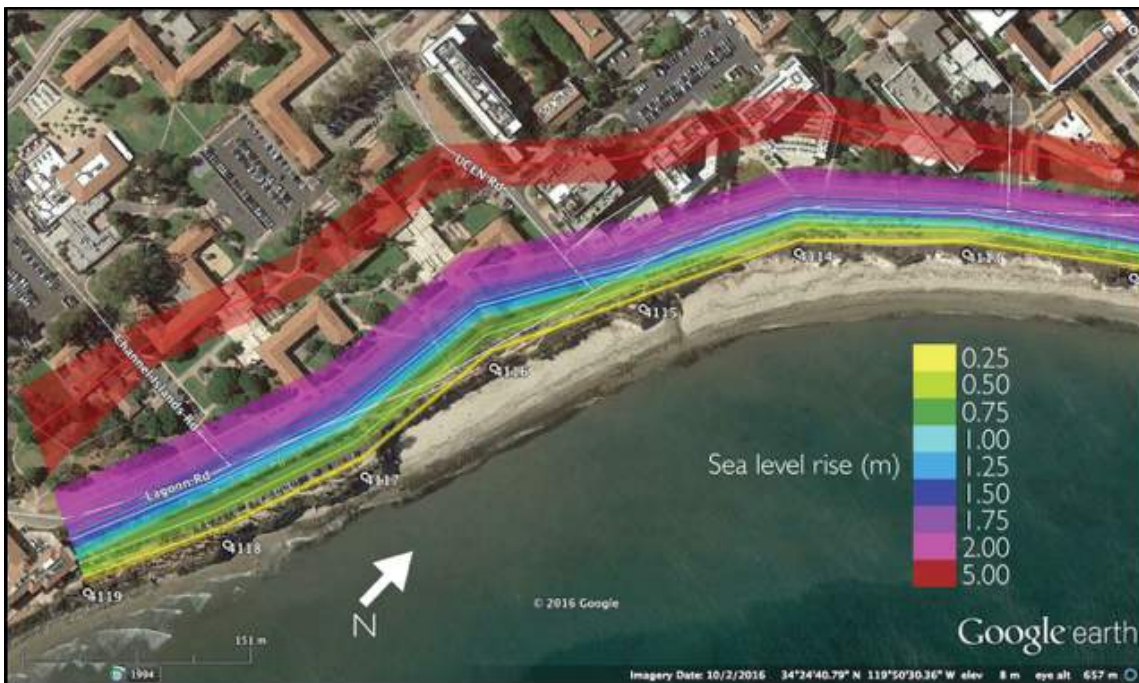
Figure 4.12. Example of cliff retreat hazards between Goleta County Beach and Campus Point. Colored bands around the lines represent projection uncertainty for that sea level rise scenario.
