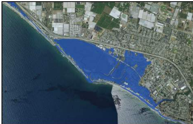
Figure 4.9. Example of future flood hazards in Goleta ( top ), Santa Barbara Harbor/East Beach ( middle ) and Carpinteria ( bottom ), showing the 1-m SLR scenario coupled with the 100-year coastal storm. See Sections 5 and 6 for salt marsh and beach ecosystem impacts.
