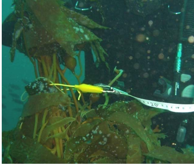
Figure 17 Twelve gauge wire and alligator clip anchoring Fish Only Transects (Photos: N. Fash, www.fashpics.com and G. Hodgson).
