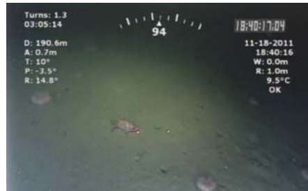
The above display is seen by operators when the ROV is in use, and this video footage is later watched by researchers who collect data on the species and habitats observed. The data is stored in a database, and the footage is archived for later use. Photo: IFAME/MARE.
